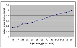
**Fig. (5)**: The relation between input energy and output energy of the thin disc laser at 1.3 kHz pulse frequency.
