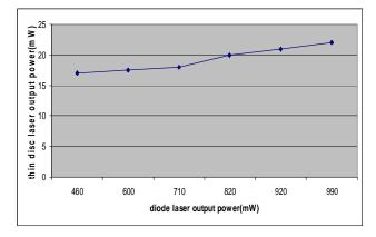
Fig. (6): Relation between the input current of pumping laser "diode laser" and output power "thin disc laser" (1064 nm)
