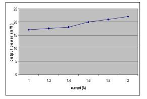
**Fig. (7):** Relation between output power of the diode laser (808 nm) "pumping power" and output power of the thin disc laser (1064 nm)
