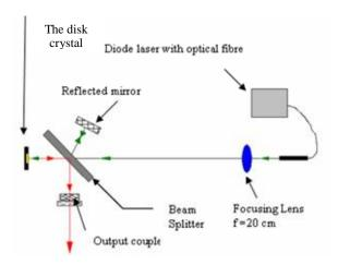
Fig. (1): Thin disc laser setup
