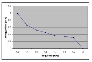
**Fig. (3):** Relation between pumping pulse Frequency and maximum output energy of the thin disc
